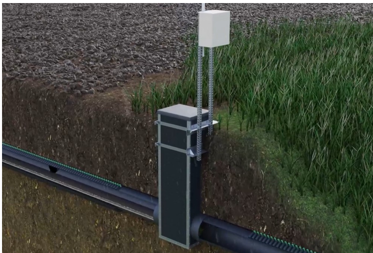
Visualization of an installed water control structure.
